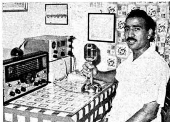
Nasin Hussain Khan, 9K2AN, of Kuwait works all bands 7-28 Mc/s running 90 watts to a Bandmaster transmitter into a dipole aerial. His receiver is a SX101.
